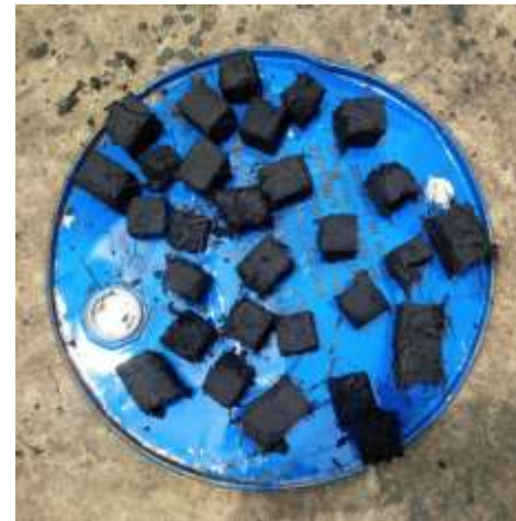
Production of charcoal briquettes from grass.
